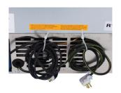
Two power cables allow refrigerator operator to select an appropriately rated available power source
